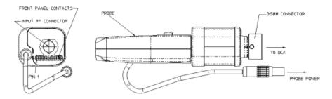
Figure 3. N1022A I/O Connections
